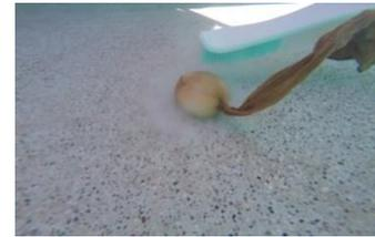
The photos below will illustrate a test showing the removal of the scale. You can see a white film that has discolored the finish. It is present on the entire pool surface. When testing an area, you can see the reaction to the topical film or calcium precipitate. Once brushed away, the calcium precipitate is removed, and your Wet Edge finish is intact below the precipitate.
